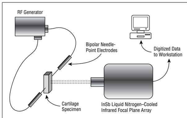
**Figure 4.** The apparatus used to measure the radiometric surface temperature of cartilage during radiofrequency (RF) heating. The indium antimonide (InSb) liquid nitrogen-cooled focal plane array was focused on the surface of the specimen between RF bipolar electrodes.
