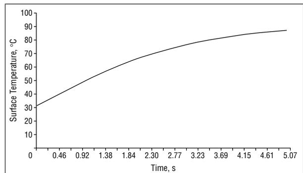
**Figure 9.** Plot depicting the average radiometric surface temperature vs time of a 1-mm-diameter area of cartilage centered in the area of maximum radiofrequency (RF) heating with the Surgitron FFPF catalog S 2100 RF generator (2.8 MHz; Elmed Inc, Addison, Ill) and bipolar needle-point electrodes.
