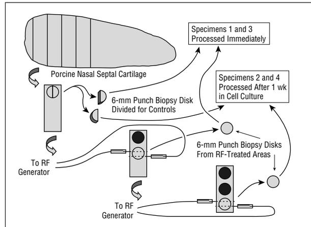
**Figure 5.** Schematic illustration of the experimental protocol used to treat cartilage specimens for chondrocyte viability determination. Two control and 2 radiofrequency-heated areas were excised by means of punch biopsy from each of 4 slabs from the cephalic end of porcine nasal septa.
