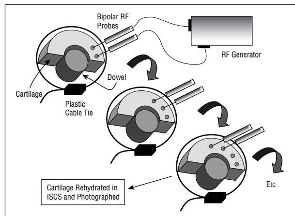
**Figure 2.** Cartilage reshaping with the Surgitron FFPF catalog S 2100 radiofrequency (RF) generator (2.8 MHz; Elmed Inc, Addison, Ill). The specimen was wrapped around a dowel and secured with a plastic cable tie. Bipolar RF electrodes were inserted and advanced in stepwise fashion, with heating of intervening cartilage at each insertion point. The cartilage was then rehydrated in isotonic sodium chloride solution (ISCS).
