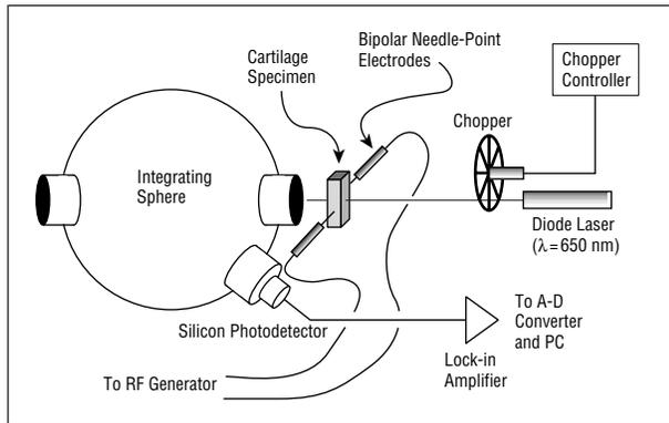
**Figure 3.** The apparatus used to measure the intensity of diffuse transmittance of laser light through cartilage during radiofrequency (RF) heating. Incident laser light is aimed at the area between the bipolar RF electrodes. A-D indicates analog-to-digital; PC, personal computer.
