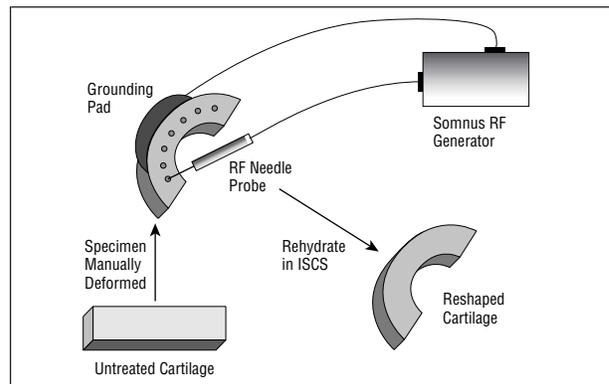
**Figure 1.** Cartilage reshaping with the model 215 radiofrequency (RF) generator (460 kHz; Somnus Medical Technologies, Inc, Sunnyvale, Calif). Manually deformed cartilage in contact with a grounding pad was heated at each electrode insertion point to a thermocouple reading of 70°C. The cartilage was then rehydrated in isotonic sodium chloride solution (ISCS).
