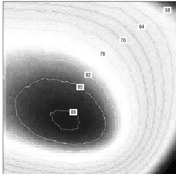
**Figure 8.** A thermal image produced using the indium antimonide liquid nitrogen-cooled infrared focal plane array. This image represents the radiometric surface temperature (measured in degrees Celsius) of a 4.5-mm<sup>2</sup> area of a cartilage specimen 5 seconds after the commencement of radiofrequency heating with the Surgitron FFPF catalog S 2100 radiofrequency generator (2.8 MHz; Elmed Inc, Addison, Ill).
