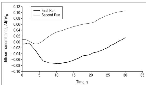
**Figure 7.** Plot depicting the diffuse transmittance ( $I(t)$ ) of laser light during radiofrequency heating. Two heating cycles are depicted. The slope of  $\Delta I(t)/I_0$  vs time reaches 0 at 4 seconds with the first cycle and 10 seconds with the second.  $I_0$  represents the signal intensity of diffused transmitted light before radiofrequency energy is applied.
